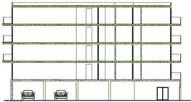
FIGURE S.0.3-1 Elevation; Simplified View of Podium Slab Supporting Four Levels of Light Framing (PTS941)
