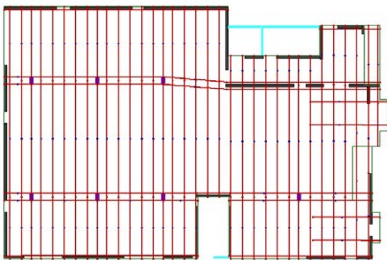
FIGURE 7.2.2-1 Plan; Arrangement of Tendons (P1357)
